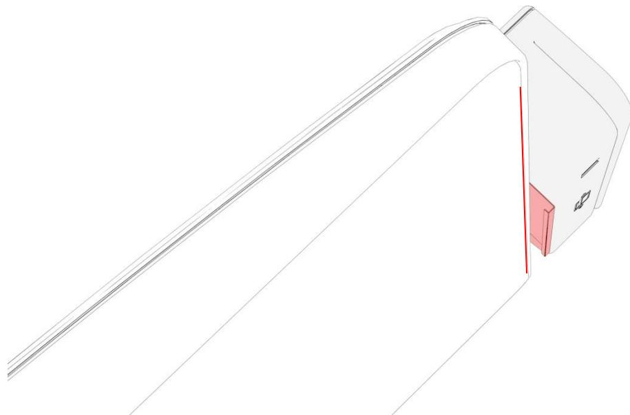
Step 4: Install the two M3 screws to fasten the MSR module.
