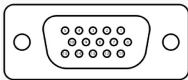
The video signal input via D-type 15-pin female connector.
