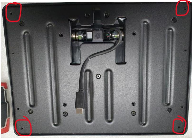
8. Attach USB-C extension cable (pn: TTETEV770014) to USB-C connector on stand, attach the other end to the USB-C port on the box pc
