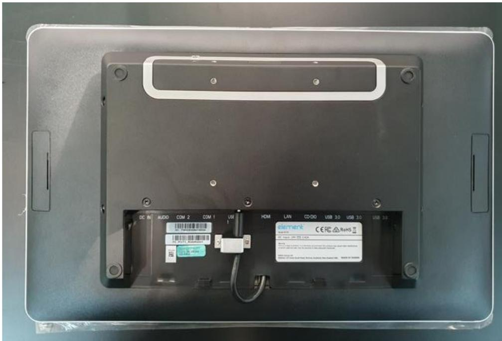
15. Reconnect power and I/O cables to box pc
