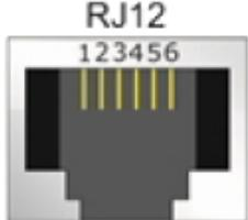
The image shows a close-up of an RJ12 connector with six pins labeled 1 through 6. The pins are arranged in a row, with pin 1 on the left and pin 6 on the right. The connector is black and white.
