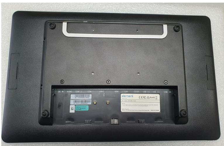
10. Re-attach USB-C cable lock to box pc and secure with the usb cable lock bracket
