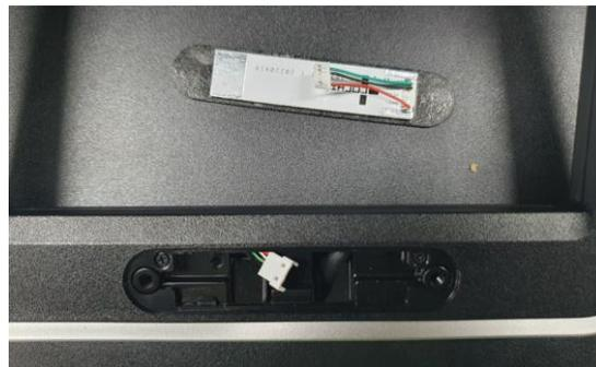
5. Connect the CDU plug to the usb connector, ensuring it is inserted squarely
