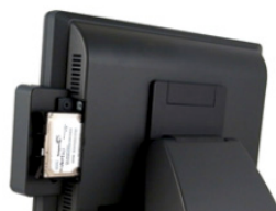
Slide in/out HDD Replacement
